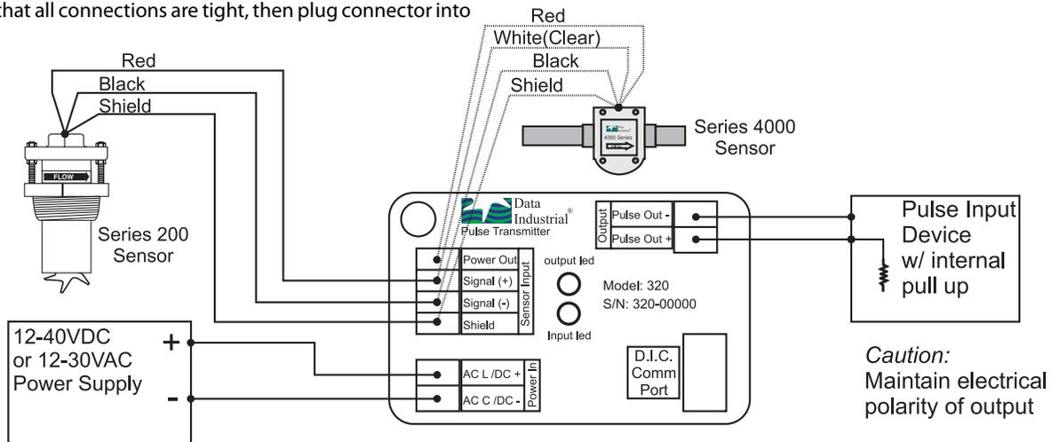
Figure 2: Typical Wiring Example
