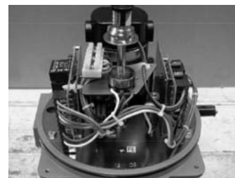
Connection to PCB Interface
