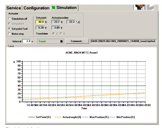
Simulation tab for damper actuators
