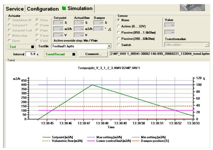
"Simulation" tab for VAV controllers
