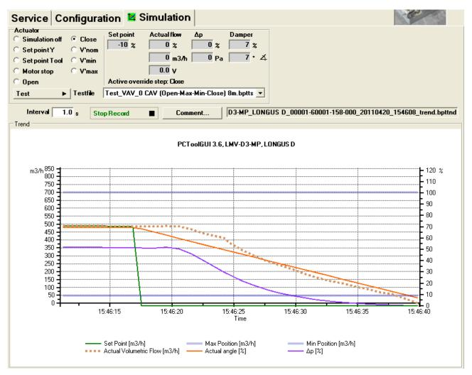
"Simulation" tab for VAV controllers
