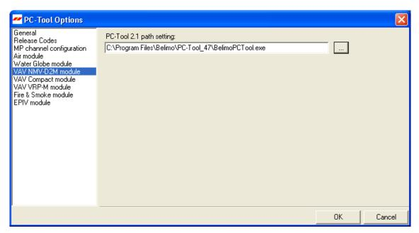
PC-Tool settings for VAV NMV-D2M module
