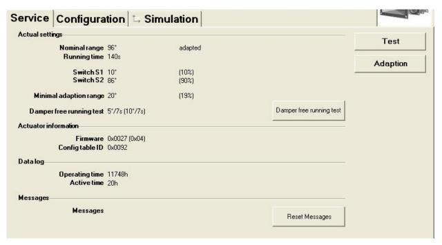
"Service" tab for BF-TopLine fire damper actuators
