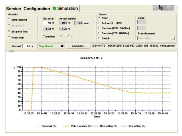
"Simulation" tab for globe valve actuators
