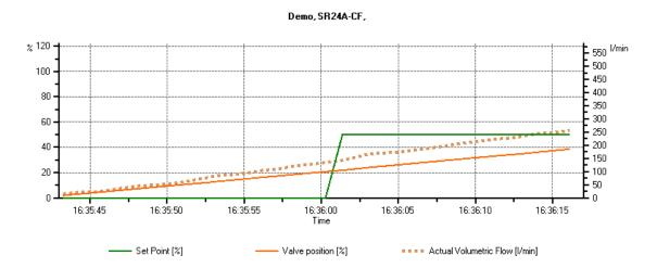
Trend diagram for the control function "Open loop"
