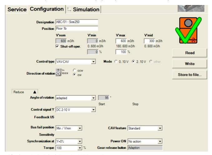
"Configuration" tab for full-rotation VAV controllers
