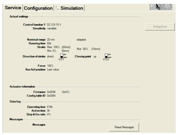
Service tab for globe valve actuators
