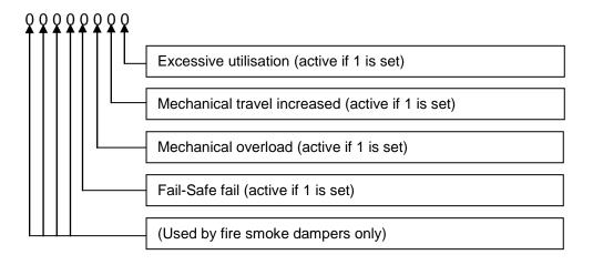
The messages can be seen in plain text in the respective PC-Tool module.
