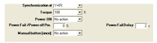
"Configuration" tab for Electronic Fail Safe (excerpt)
