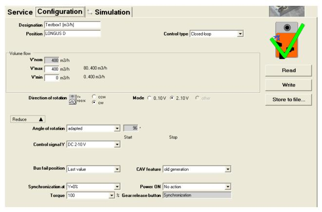
"Configuration" tab for full-rotation VAV controllers
