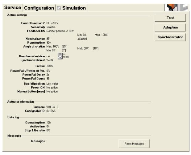
Service tab for full-rotation damper actuators
