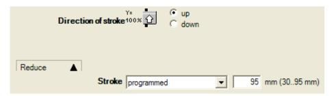
"Configuration" tab for linear actuators (excerpt)
