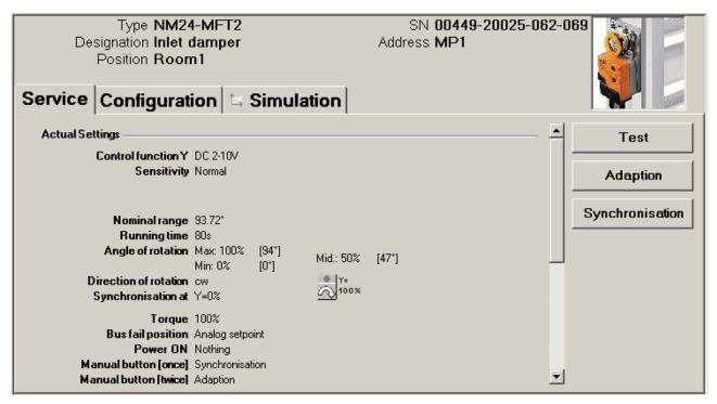
Example of detail area [D] (damper actuator)
