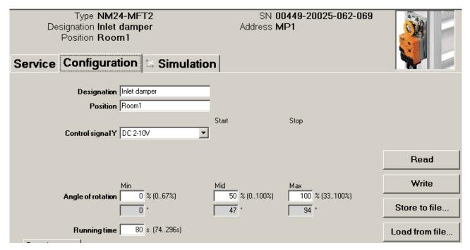
Example of the "Configuration" tab (damper actuator)
