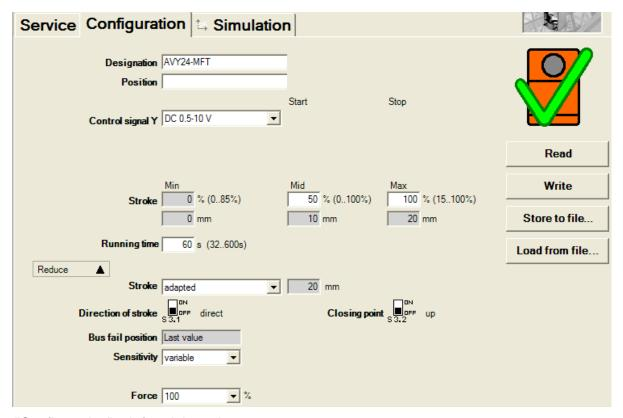
"Configuration" tab for globe valve actuators
