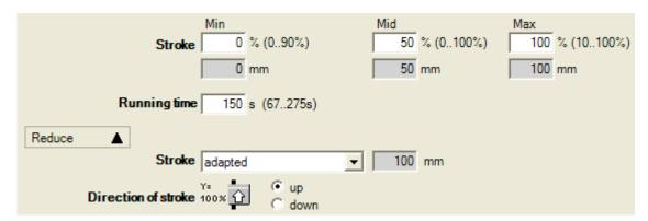
"Configuration" tab for linear actuators (excerpt)
