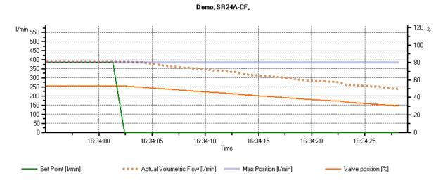
Trend diagram for the control function "Flow control"
