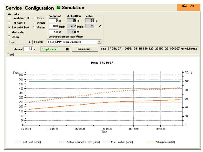
"Simulation" tab for VAV controllers
