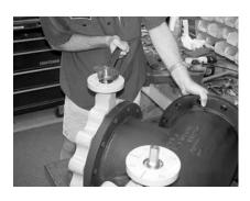
Step 2) Referring to the three configuration types on page 3 of the SY IOM, position the master and slave valve discs as instructed. For example, if you have a configuration code X20 tee assembly, you will OPEN the Master valve (M) and CLOSE the Slave valve (S).
