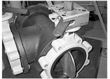
Step 3) Install the MASTER valve crank arm onto the MASTER valve in the correct orientation, as shown. Install the SLAVE valve crank arm onto the SLAVE valve in the correct orientation, as shown.
