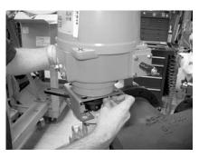
Step 14) Stand with the opening in the actuator bracket facing towards your LEFT. Hold the SY actuator with the handwheel on the RIGHT, and the EMT connectors to your LEFT. Align the square drive or keyway in the SY
