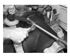
Step 26) Once the SLAVE valve has been determined to be in the correct position, lock the jam nut against one of the yoke ends to prevent any changes in the adjustments just completed.
