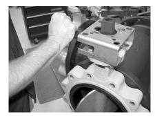
Step 8) To facilitate the insertion of the mounting bolts, it may be necessary to move the valve disc, and therefore the crank arm, to gain access to the mounting holes.
