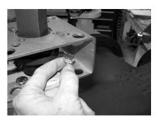
Step 7) Insert the four bolts and mount the bracket to the valve mounting flange. Attach the lock washers and nuts, but do NOT tighten at this time.
