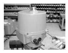
Step 2) Remove cover from the SY actuator. A flat blade screwdriver inserted carefully into the provided slot (as shown) will facilitate removal of the cover.
