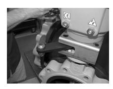
Step 20) With the MASTER valve in its fully OPEN position and the SLAVE valve in its fully CLOSED position, assemble the yoke and clevis pins onto the crank arms, pointing towards each other as shown.
