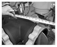
Step 21) Measure the distance between the inboard end of the yokes to determine the proper length of the connecting rod. It is important to make sure the MASTER and SLAVE valves are in their proper positions (OPEN and CLOSED, respectively) before
