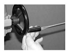
Step 12) Attach the hand knob to the hand wheel as shown below (if not already completed).
