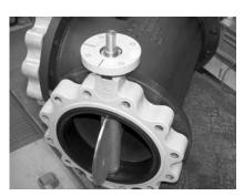
Step 1) Both valves must be stripped down to their basic form. Remove all other linkage components before starting the assembly sequence below. The linkage components have been designed to attach to the valves in their basic form state rather than to any existing hardware.
