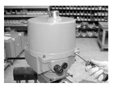
Step 2) Remove cover from the SY actuator. A flat blade screwdriver inserted carefully into the provided slot (as shown) will facilitate removal of the cover.
