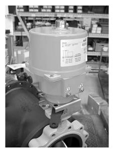
Step 18) When mechanical assembly is complete, the SY actuator and MASTER valve should be oriented as shown below. The actuator is in the OPEN position, and the valve disc is fully OPEN, and all bolts are tight.
