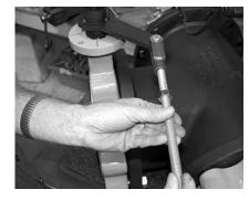
Step 22) After the connecting rod is cut to the correct length, screw it into SLAVE valve yoke end until the threads pass through the yoke and just start to protrude into the inboard end of the yoke. The rod lock nut should be closest to the SLAVE valve yoke end.
