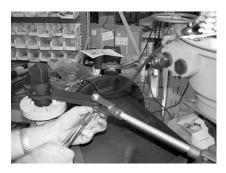
**Step 27)** Insert two cotter keys into the two clevis pins.
