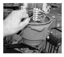
Step 6) Apply proper voltage to terminals #1 (Neutral) and #7 (Hot). Apply proper actuator voltage to terminals #1 (Neutral) and #4 (Hot) to drive the actuator CLOSED until the end-of-travel cam STOPS the actuator movement. (Note that there is no terminal #2).
