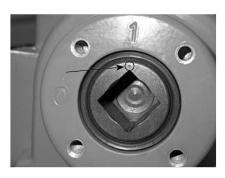
Step 11) Verify that the SY actuator is in the OPEN position also by looking at the bottom of the actuator. There is a dimple mark punched in the output shaft which will align with the "1" mark when the actuator is in the OPEN position.
