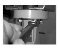
Step 17) Now tighten the four bracket bolts (B, C, D) assembled in step 6 above.
