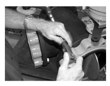
Step 23) Remove the MASTER valve yoke end and thread it onto the connecting rod. Adjust the distance between the yoke centers to match the hole in the MASTER valve crank arm.
